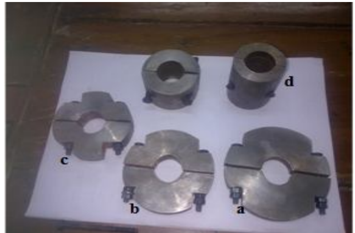
Fig. 3: Rotor disks, (a) 100 mm outer diameter & thickness 12.5 mm, (b) 90 mm outer diameter & thickness 15 mm, (c) 80 mm outer diameter & thickness 20 mm, (d) 50 mm outer diameter & thickness 60 mm
